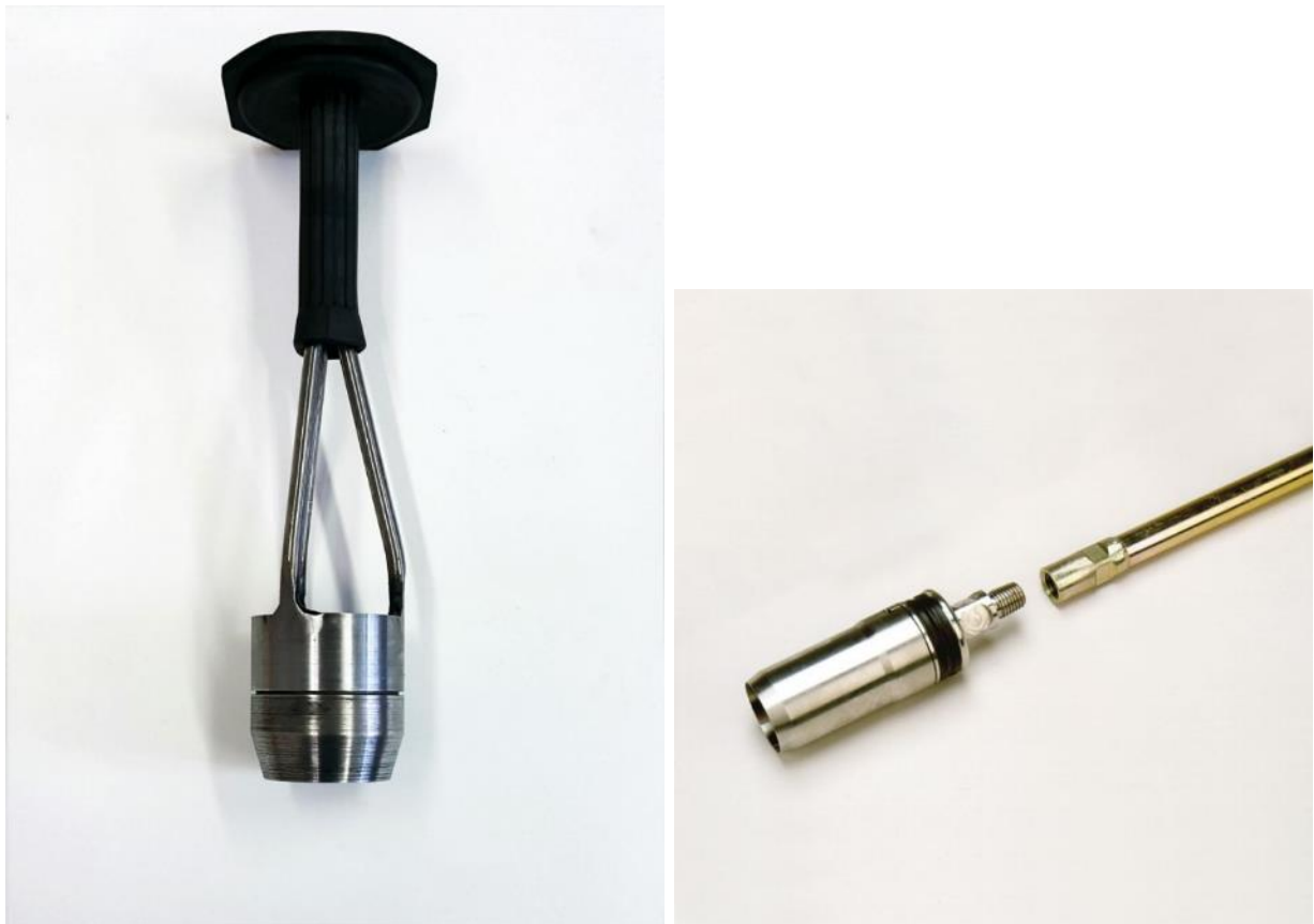
Figure 12: Examples of ring samplers for bulk density.
