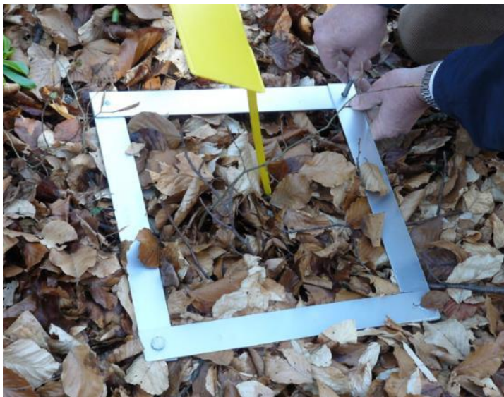
Figure 10: Example of a frame for collecting litter.
